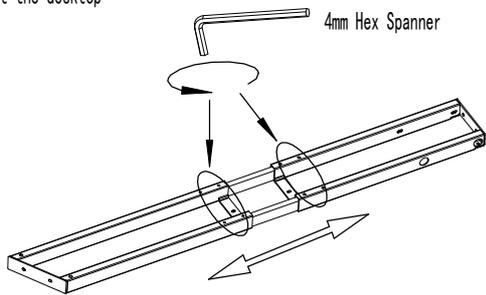
**2** Attach legs to the beam using 4 of M6\*14 screws and 2 of M6\*12 screws
