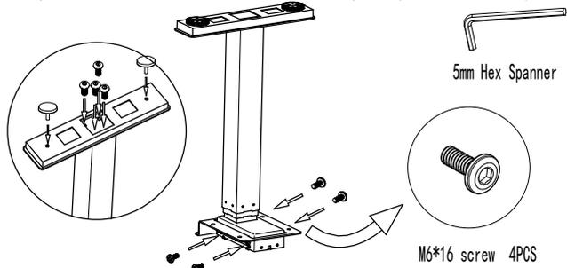
**6** Attach connection fittings to beams using 4 of M8\*10 screws
