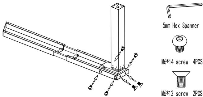
**3** Attach feet to the legs using 4 of M8\*16 screws, attach the 2 of levelling foot pads to the feet by hand
