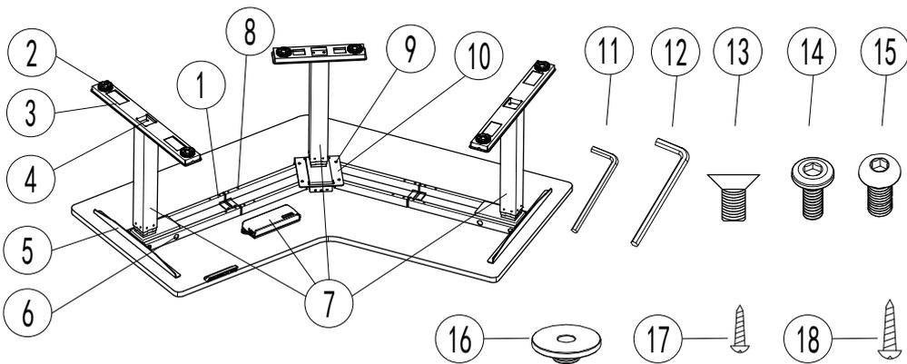
**1** Loosen the 4 screws of beam using 4MM hex spanner, adjust the beam to proper position to fit the desktop
