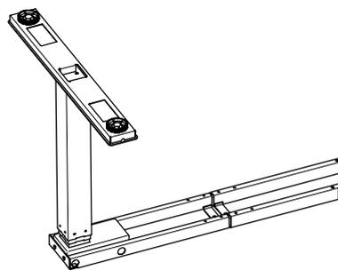
**5** Attach legs to connection fittings using 4 of M6\*16 screws, attach feet to the legs using 4 of M8\*16 screws, attach the 2 of levelling foot pads to the feet by hand
